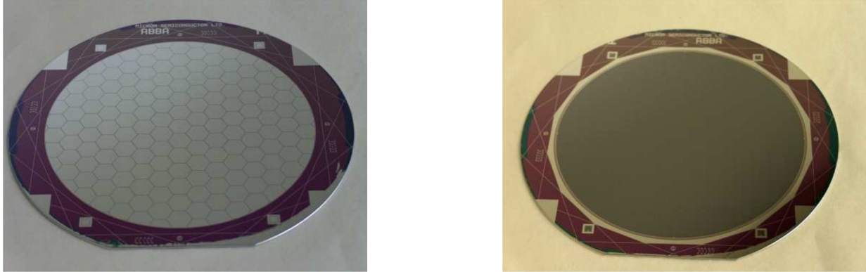
Figure 8: Photographs of the prototype abBA/Nab detector, before cutting from the 6 inch diameter silicon wafer and packaging. Charged particles enter through the junction side (left) and signals are read out from the ohmic side(right).
