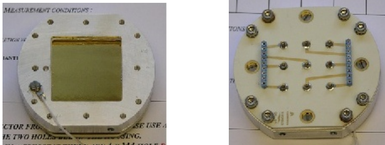
Figure 10: The view of the front side (left) and back side (right) of the 9 cm 2 segmented Si(Li) detector. All nine contacts, one per segment, can be seen on the back.
